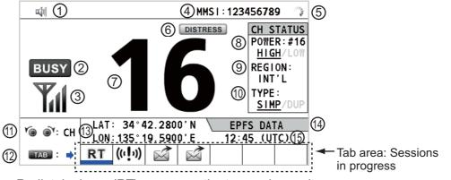
Radiotelephone (RT) screen on the transceiver unit
